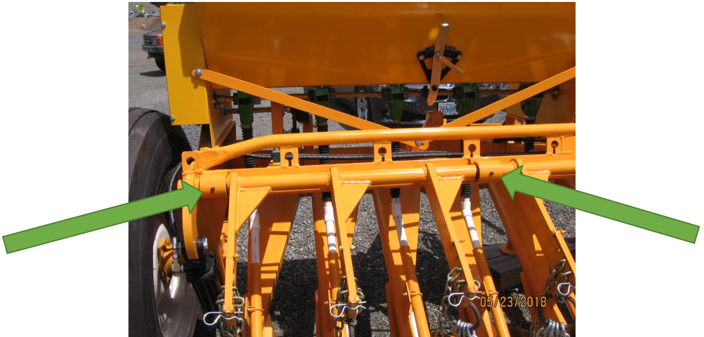
SLEEVE HINGES SUPPORTING THE OPENER ARM ASSEMBLIES GREASE ZERK (5 TOTAL)
