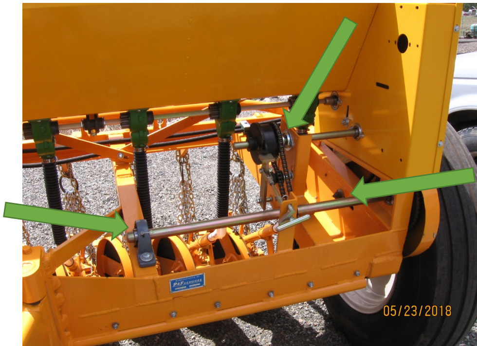
SEED BOX ACTUATING MECHANISM GREASE ZERKS (3 ON EACH SIDE)
