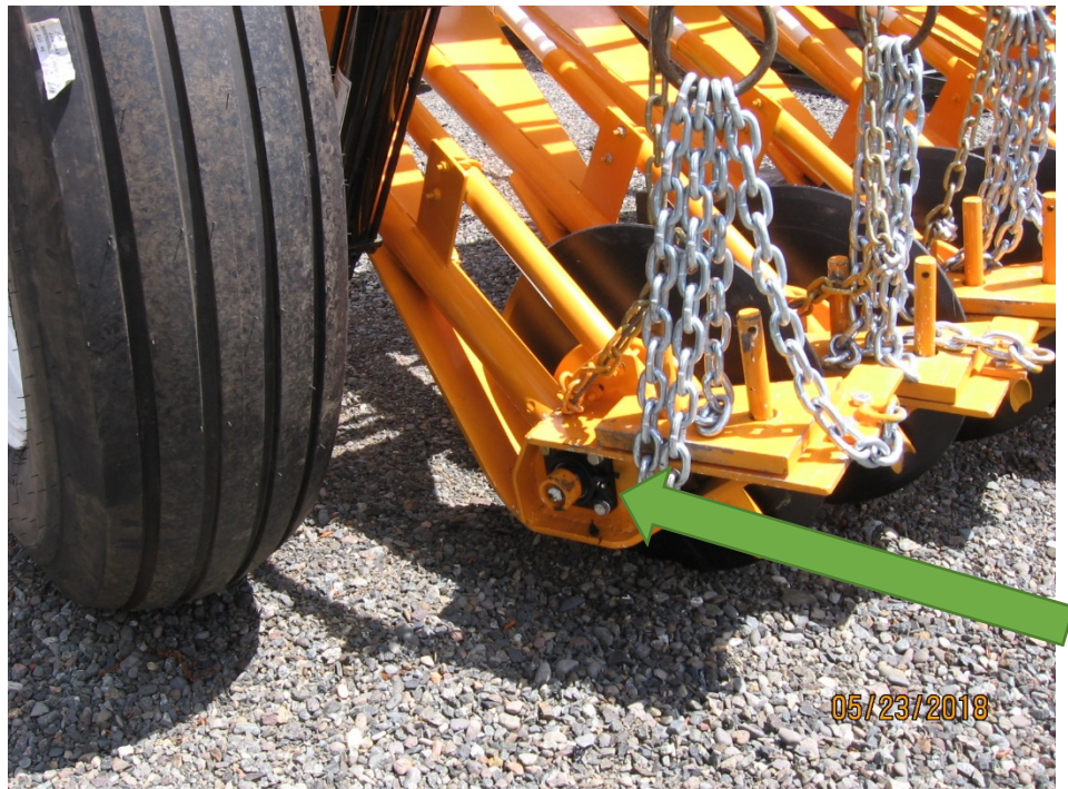
DISK OPENER GREASE ZERK LOCATION (10 TOTAL)
